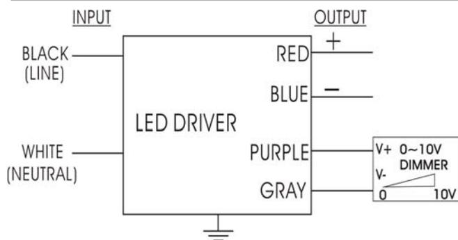
Maximum Wiring Distance(at full load) is 18AWG/18Feet
