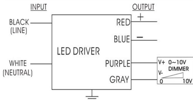
Maximum Wiring Distance(at full load) is 18AWG/18Feet
