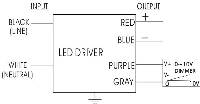
Maximum Wiring Distance(at full load) is 18AWG/18Feet
